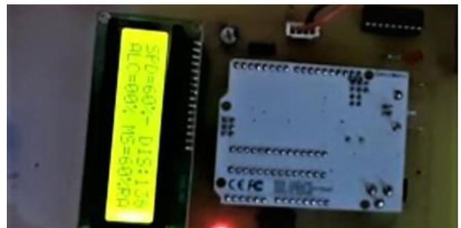
Figure 6. Result for Blind Radio Frequency is activated and max speed limit is 60% when accidental zone is detected
