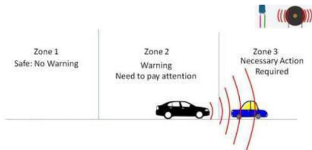
Figure 2. Creating accidental zones to detect front vehicle warning.
