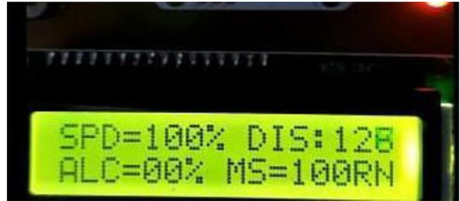
Figure 8. Result of speed, distance, alcohol and Rf signal is showing in LCD display
